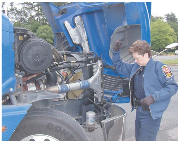
Police officer Sally McGowan, with the Motor Carrier Safety Unit, examines the suspension, brake chamber and leaf spring of a Sunoco fuel truck from Philadelphia. If the leaf spring's U bolts are loose, the axle will shift, causing a dangerous condition.
