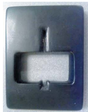
A skimmer removed from the ATM machine located in the lobby of the Inova Fairfax Hospital Cardiac Care Center.
