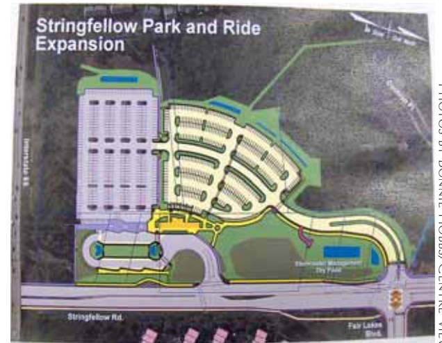
Site plan of the park-and-ride expansion. The new parking spaces are in yellow.
