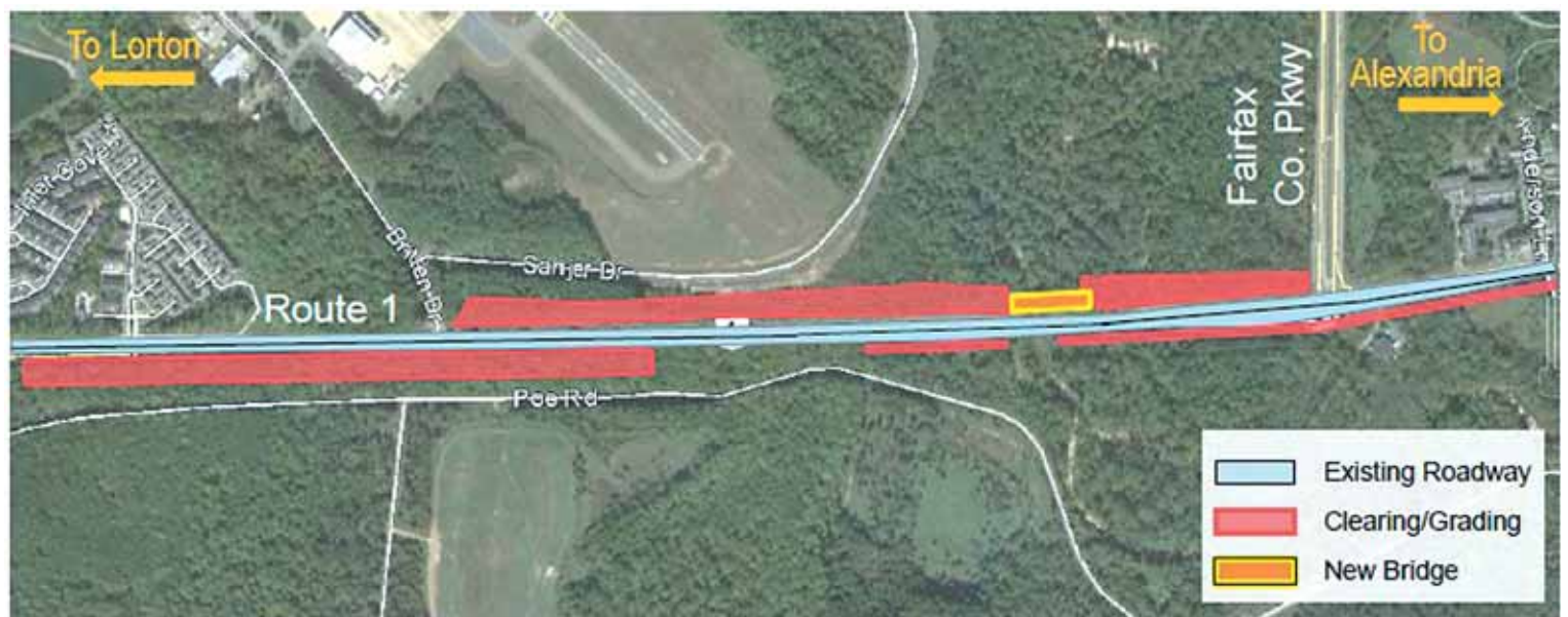
Section B of the U.S. Route 1 Improvement project, showing clearing and grading taking place, as well as the location of the new bridge over Accotink Creek.
