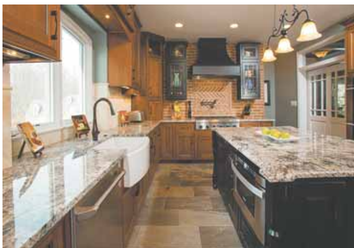
The bow front farm sink, six-burner stove and food prep island form the three sides of a work triangle that facilitates cooking and clean-up tasks. The custom-designed barn door (right) leads into the new formal dining room.
