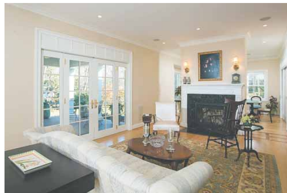
The split-level’s former bow window was converted to a set of French doors which overlook the new veranda. Though the execution makes the addition hard to detect, the dining room beyond the fireplace is actually in the home’s new wing.
