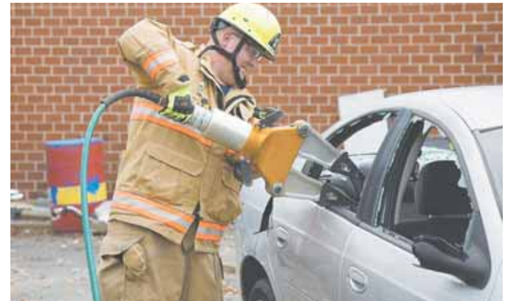
Joel Fry, a master technician with the station, operates the Jaws of Life hydraulic tool during a vehicle extrication exercise for open house spectators. When car accident victims cannot be removed safely from a vehicle, firefighters are trained to remove doors, the roof and the dashboard of a vehicle to make more room for paramedics and EMTs.
