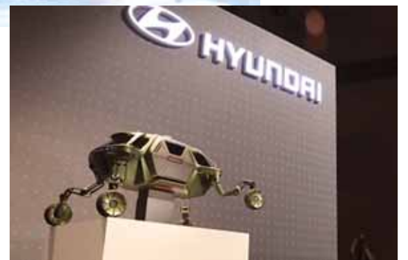
The Hyundai Elevate, a concept vehicle dubbed the "walking car," uses articulated legs to navigate off-road following floods, fires, earthquakes and other natural disasters.
