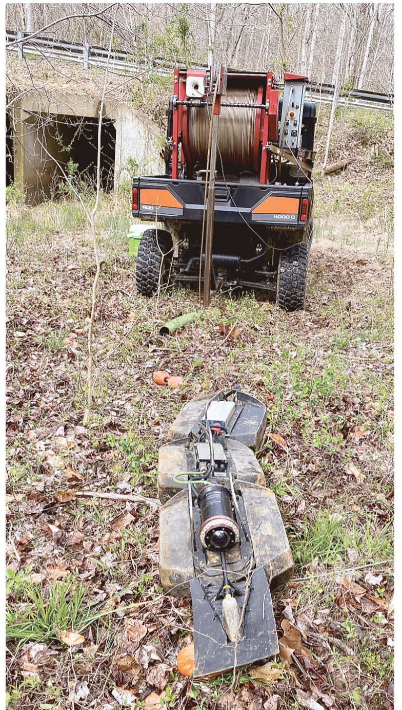
Robot equipped with camera ready to video pipe conditions.
