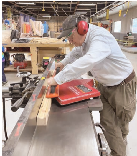
MERCIA HOBSON/CONNECTION NEWSPAPERS Safety goggles and ear protectors are in place as Randy Hill prepares a board on the jointer.
