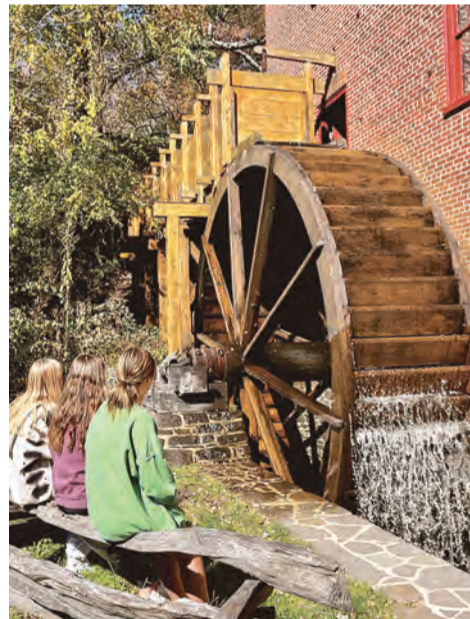
Local teens (from left) Elizabeth Hanes, 17, of Herndon, Reese Higgins, 14, of Great Falls, and Elizabeth Crawford, 12, of McLean, watch the water having dropped into the flume and through the sluice gate, begin filling the buckets on the 20-foot waterwheel. The wooden power shaft is attached to the waterwheel and powers the mill.
