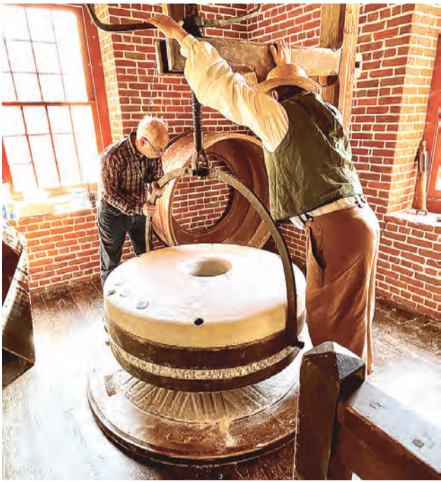
(Right) Steve Golobic, miller at Colvin Run, and volunteer Bob Coblerz of Springfield set the millstones in place during Harvest Time at Colvin Run Mill.
