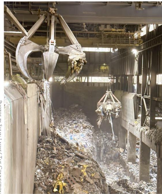
Overhead grapple cranes operate on sliding gantries moving large quantities of trash to begin the combustion process.
