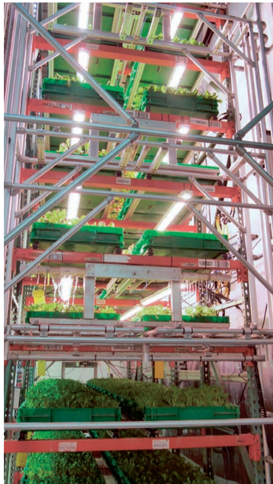
Area 2 Farms uses a patented process using rotating trays for indoor plants to simulate a 24-hour cycle.
